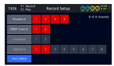
**Record Setup:** Mesa will default to automatically select which channels to record on the microSD card based on whatever inputs are connected at the time of the recording. If one wishes to manually specify which input channels are to be recorded, that can be selected on the Record Setup page. Choose from any combination of Preamp, SPDIF Coax, Loopback and Optical channels.
