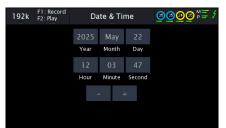
**Date & Time**: Set the Internal Mesa clock, which is used to timestamp microSD card recordings. When using Mesa Remote, you can have the computer date and time sent down to the Mesa to set this value. See section 4.1.
