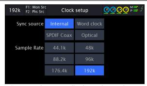
This page is where we set the **Sync Source**, and can manually change the sample rate. Sync Sources are only selectable here when they are valid. For instance, unless the SPDIF coax input is connected to a device's SPDIF output, SPDIF Coax will not be a selectable option. The same is true for Wordclock and Optical. Internal is when the Mesa operates from its own high-quality crystal oscillator clock. That is the default, and, in most cases, the ideal choice.
