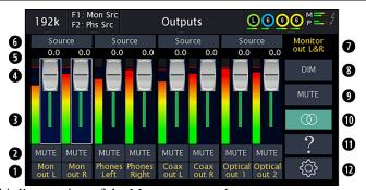
This page is where you get a bird's eye view of the Mesa outputs, where you can attenuate outputs, assign sources, and control other parameters. Many users will monitor input signals through their recording software, and, likely, will not need to make changes from the defaults. However, if users want to do zero-latency hardware monitoring, or set up mirroring of signals to multiple outputs, or other more advanced functions, this is a good starting place to make those changes.
