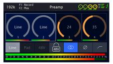
When Hi-Z is the selection for an input, pad and 48V do not apply and will be grayed out.
