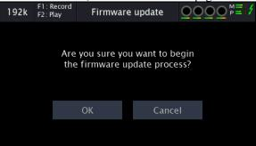
After pressing the OK button, the firmware update will progress through the same four stages described in the previous section: Erasing, Programing, Verifying, Complete. When programming is complete, you will be prompted to power down the Mesa using the back panel power switch. After doing so, the new firmware will be active.
