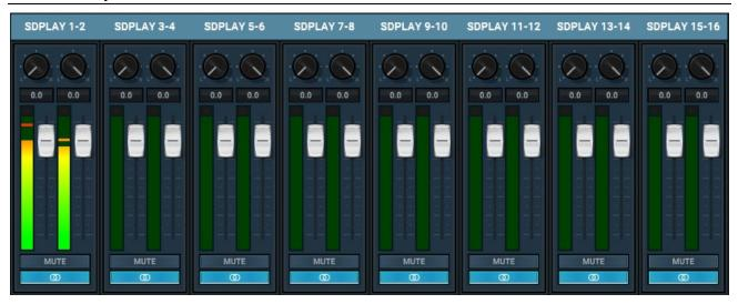
Above the Outputs pane is the SD Play pane. This is where tracks that have been recorded onto a microSD card can be directed to any outputs on the Mesa. By default, the SD card tracks will play through the Monitor and Phones output, but you can customize it if you wish to.
