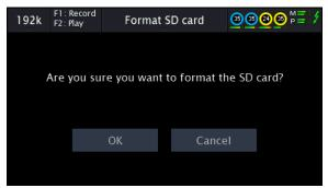
**Format:** This is a handy place to format a microSD card using the recommended ex-FAT formatting method. It is recommended to re-format the microSD card after transferring audio from the card to a computer. Many current operating systems write files to a card when data is pulled off of it, and these files can corrupt future recordings. After transfer, reformat before starting a new recording in the Mesa.
