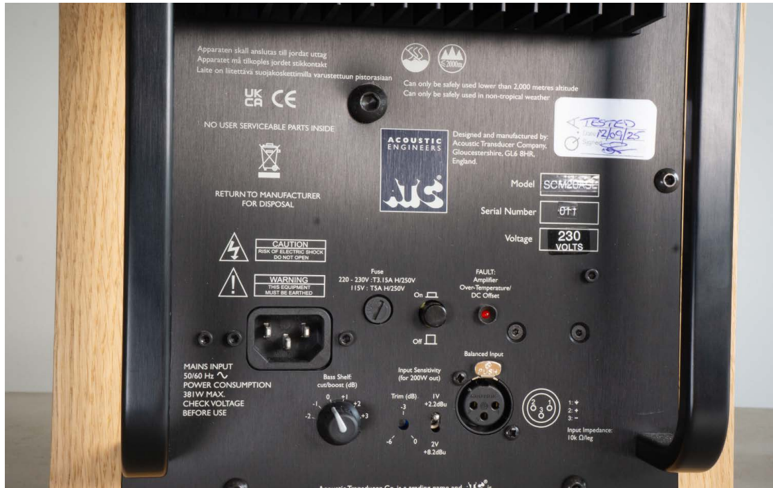
Rear panel inputs and controls with mains and signal input (XLR), power on/off, sensitivity and bass adjustment controls
