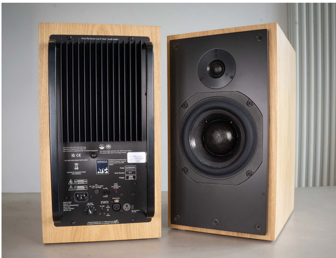
Rear panel showing the amp pack controls and substantial heatsinking
